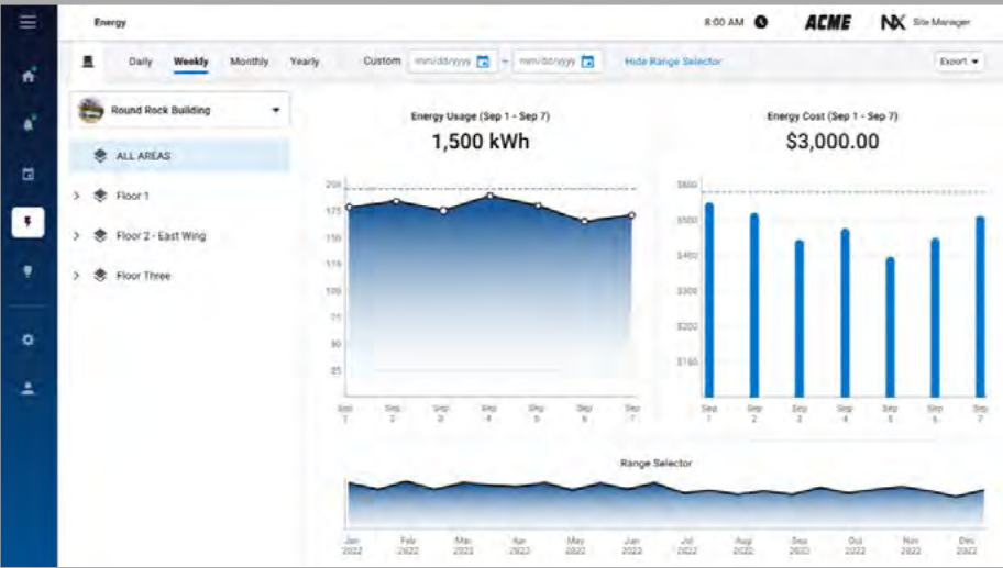
View Lighting Energy Usage in Energy Dashboard
