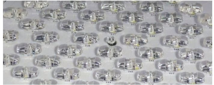
Encapsulation construction of LED Arrays
